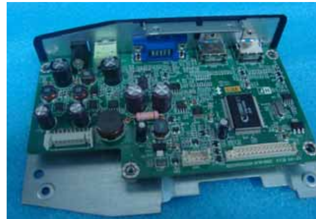
S8: Assemble the chassis and the main board
